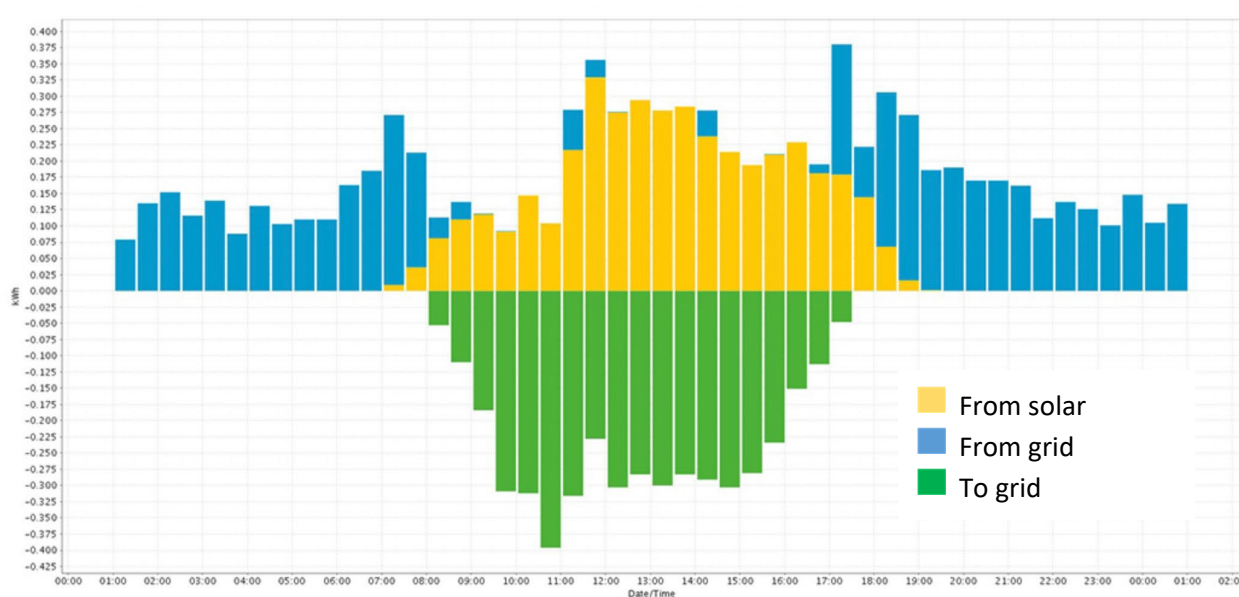
Figure 36. More complete information on solar and load possible with solar PV production meter [50].
